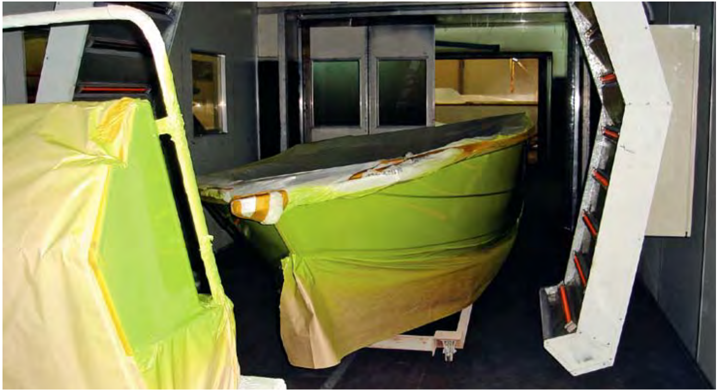
Above: My freshly painted rig about to enter the Stargate to be transported to another dimension. Actually it's in the drying oven where the paint is baked to a tough, shiny finish. The tape job minimises the chance of overspray creeping on to white hull.
