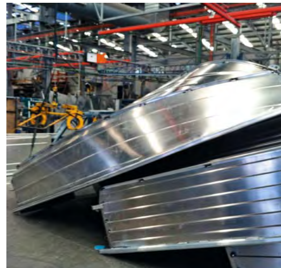
Above: This must be how Stacers reproduce in their natural environment. The steeply raked forefoot, which is part of the EVO Advance hull concept, softens the ride in choppy conditions.
