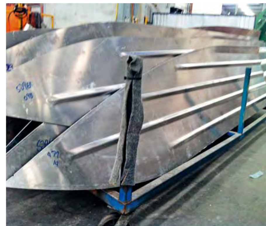
Below: Someone with a really big can opener has taken to a really big sardine can and ended up with these nifty hull panels. Note the pronounced reverse chine (top right) which aid stability.
